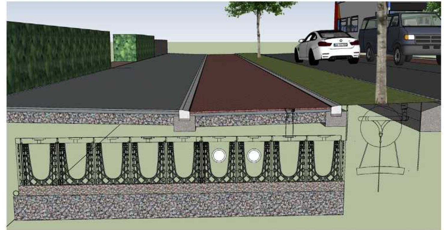
Indicative arrangement of tree in grass verge with Rootsace System
