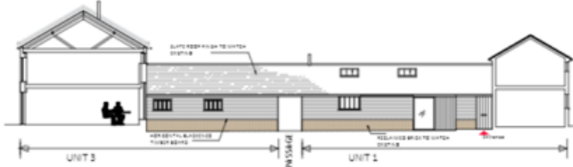
2 NORTH ELEVATION- COURTYARD
